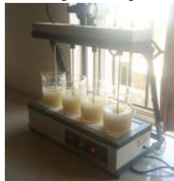
Fig.4: Jar test apparatus
